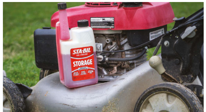
A fuel stabilizer can be added to gas-powered tools if you plan to leave gas in the tank over the winter.
